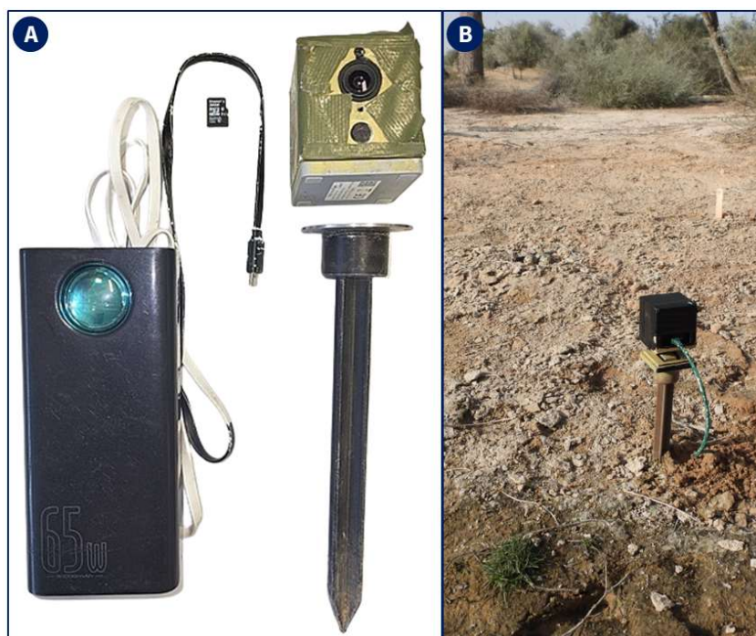
Figure 7: A) Complete system for recording behaviour at the nest: power bank, power cable, microSD card, camera and stand; B) camera installed beside a nest.
