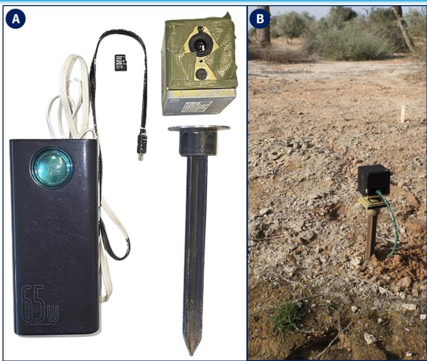
Figure 12: A) a complete set for recording nest behaviour: a powerbank, power cable, microSD card, camera, and stand; B) installation of the camera near the nest.
