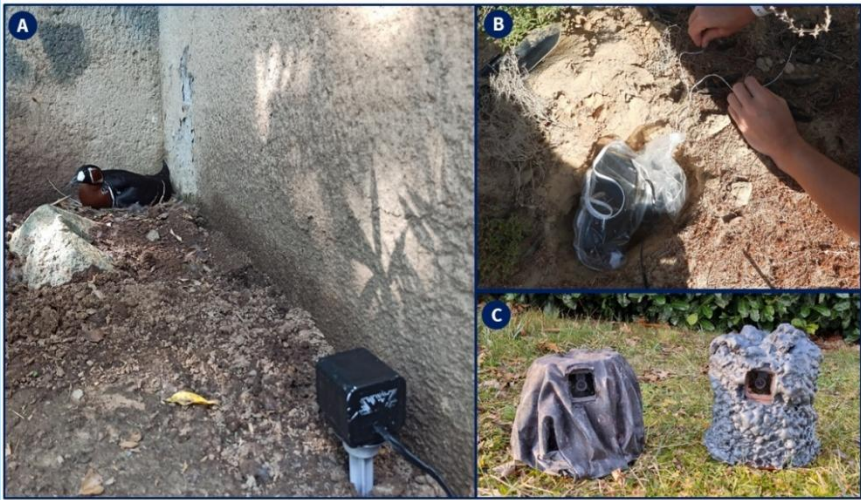
Figure 11: A) the camera in the enclosure, B) the powerbank hidden in the substrate, C) the camera placed in a fake stone.
