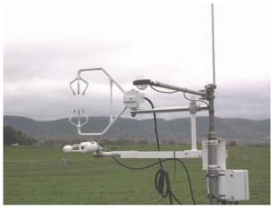
Figure 6.5 Solar-powered climate stations equipped with data loggers (left) are used to provide data (wind speed, air temperature, humidity) to support computations of snowpack convective exchange. The addition to climate stations of sonic anemometers (top right), fine-wire thermocouples, and high-speed open-path gas analyzers for  $\rm CO_2$  and water vapor (bottom right) allows computation of convective exchange using the eddy covariance method (photographs by D. DeWalle).
