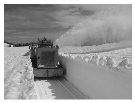
Figure 1.5 Transportation department snow blower at work clearing Highway 143 between Cedar Breaks and Panguitch, Utah in 2005. (Courtesy R. Julander.) See also color plate.
