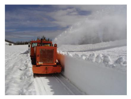
Figure 1.5 Transportation department snow blower at work clearing Highway 143 between Cedar Breaks and Panguitch, Utah in 2005. (Courtesy R. Julander.)
