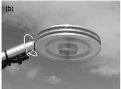
Figure 4.6 Hotplate snow gauge operation where both upper (a) and lower (b) plates are heated and maintained at 75 °C. The power difference between the top and bottom plates is proportional to the precipitation rate (courtesy R. Rasmussen, National Center for Atmospheric Research).
