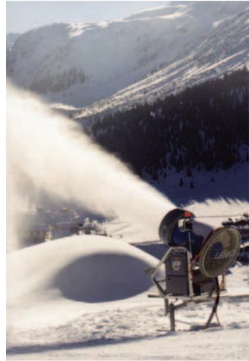
Figure 12.11 Ratnik low-energy modified snow gun (left) and modified fan-type Lenko snow gun (right) being used to augment snowpack for skiing (courtesy of Ratnik Industries, Inc. and Lenko Quality Snow, Inc., respectively).
