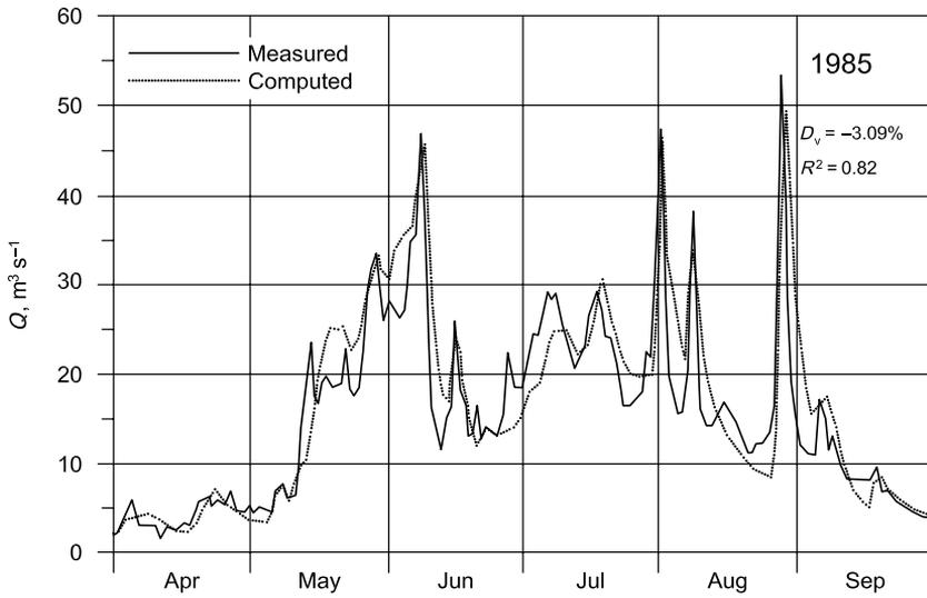
Figure 11.14 Runoff simulation in the catchment area of the hydroelectric station Tavanasa (Swiss Alps, 215 km<sup>2</sup>, 1277–3210 m a.s.l.) (Baumann *et al.*, 1990, courtesy K. Seidel).
