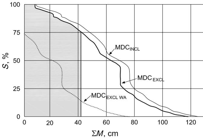
Figure 11.24 Modified depletion curves for zone A:  $MDC_{INCL}$  derived from CDC, therefore including new snow,  $MDC_{EXCL}$  with new snowmelt excluded,  $MDC_{EXCL WA}$  with “winter deficit” (shaded area) cut off.
