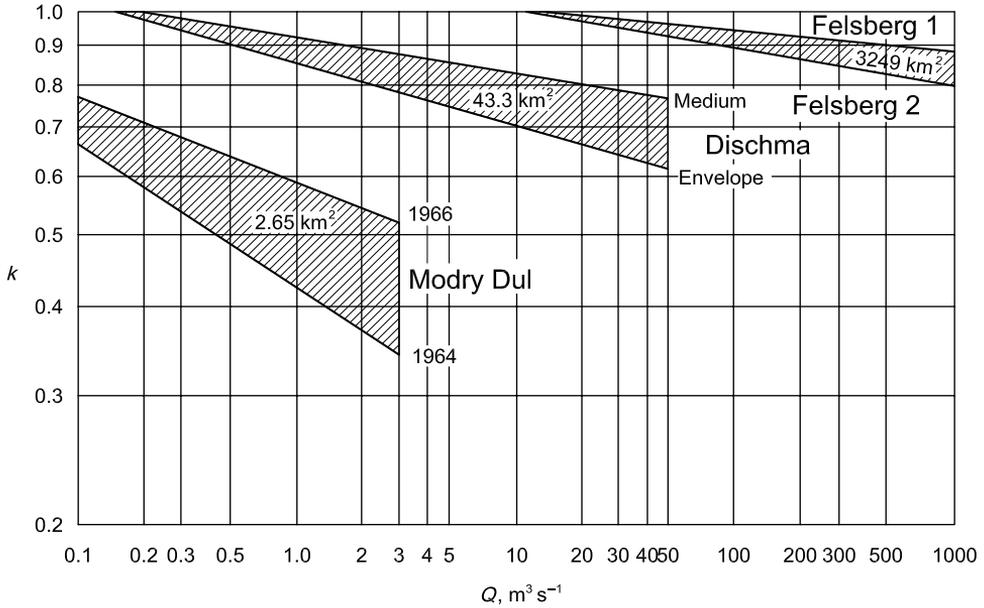
Figure 11.10 Range of recession coefficients,  $k$ , related to discharge  $Q$  resulting from various evaluations: In Dischma, the range results from using either the envelope line or the medium line in Figure 11.9. In Modry Dul, the relation varies in different years. In Felsberg, the relations (1) and (2) are derived from the size of the basin by two alternative formulas (Martinec and Rango, 1986).
