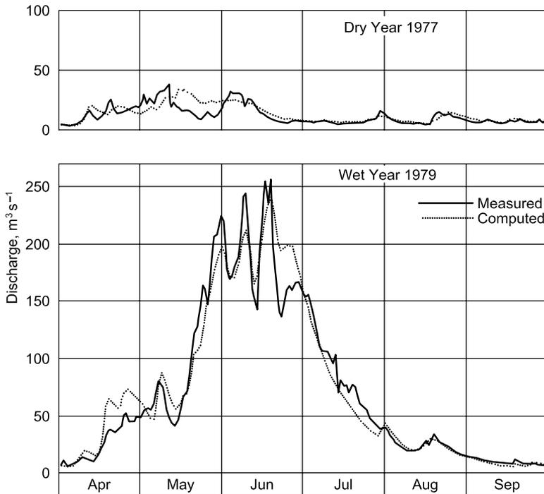
Figure 11.12 Runoff simulations in the basin of the Rio Grande near Del Norte, Colorado (3419 km<sup>2</sup>, 2432–4215 m a.s.l.) (Martinec and Rango, 1989).
