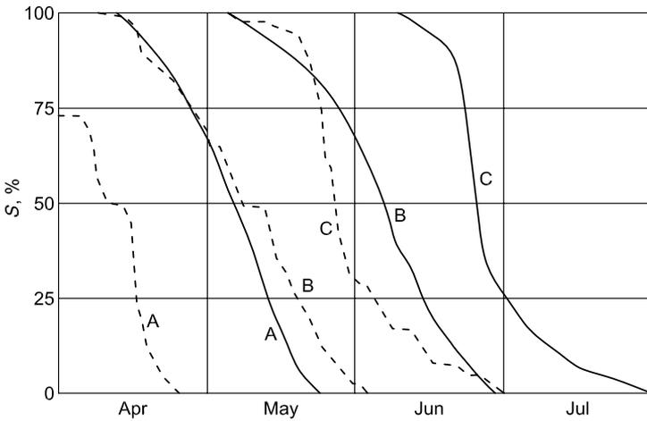
Figure 11.27 Effect of a changed climate ( $T + 4\text{ }^{\circ}\text{C}$ ) on snow-covered areas of 1979 in elevation zones A, B, and C of the Rio Grande basin near Del Norte.  $CDC_{CLIM WA}$  is shifted from the original CDC due to a reduced snow cover on April 1 and due to increased temperatures in the snowmelt season.
