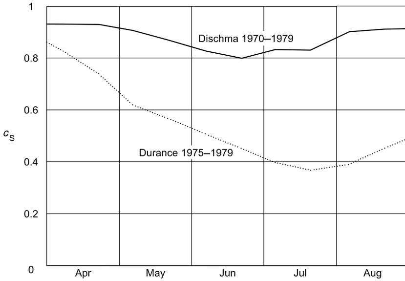
Figure 11.6 Average runoff coefficient for snow ( $c_s$ ) for the alpine basins Dischma (43.3 km<sup>2</sup>, 1668–3146 m a.s.l.) and Durance (2170 km<sup>2</sup>, 786–4105 m a.s.l.) (Martinec and Rango, 1986).
