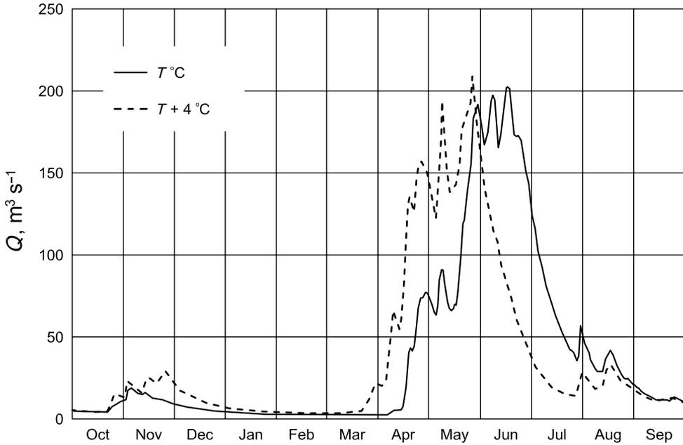
Figure 11.29 Simulated runoff in the Rio Grande basin near Del Norte in the hydrological year 1979 and climate-affected runoff computed by increased temperatures ( $T + 4\text{ }^{\circ}\text{C}$ ) and correspondingly changed snow conditions.
