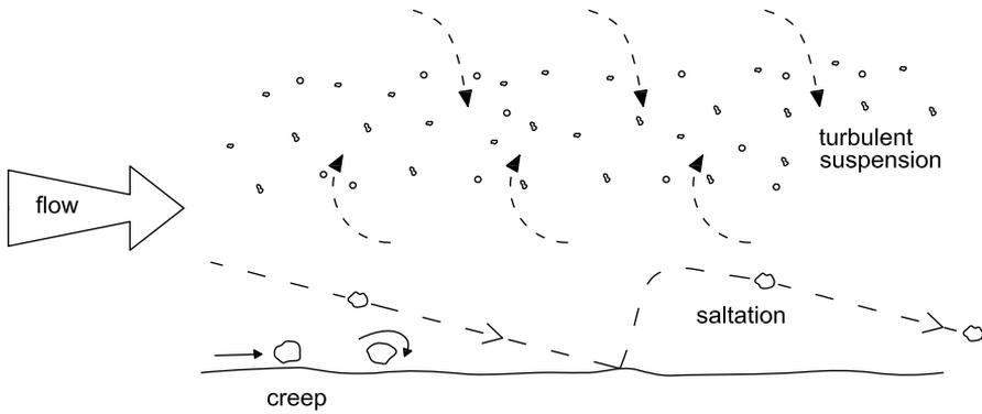
Figure 2.11 Modes of transport for blowing snow.
