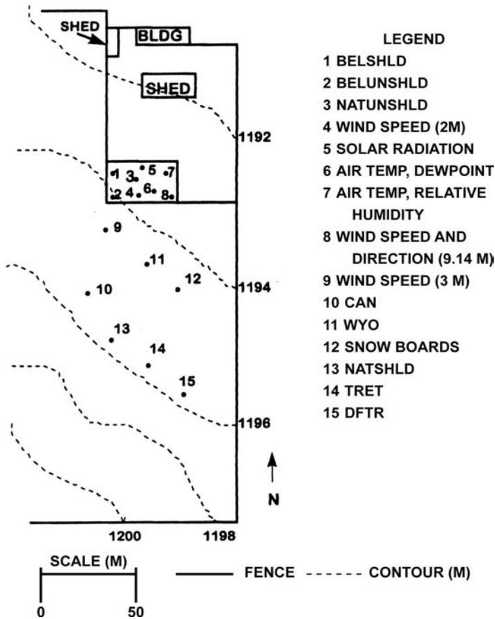
Figure 4.4 Location of precipitation gauges and other meteorological instrumentation on the RCEW test site (adapted from Hanson *et al.* [1999]).
