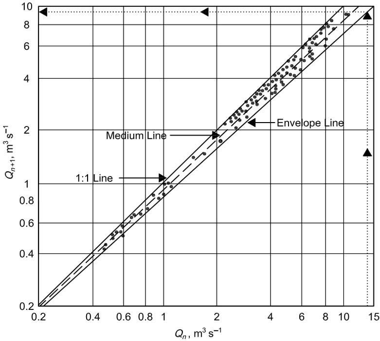
Figure 11.9 Recession flow plot  $Q_n$  vs  $Q_{n+1}$  for the Dischma basin in Switzerland. Either the solid envelope line or the dashed medium line is used to determine  $k$ -values for computing the constants  $x$  and  $y$  in Equation (11.7) (Martinez and Rango, 1986).
