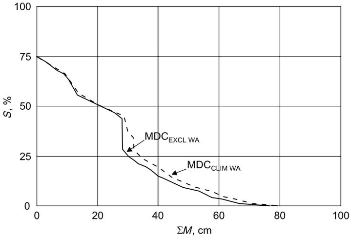
Figure 11.26 Modified depletion curve, adjusted for the “winter deficit” and including new snow of the changed climate ( $MDC_{CLIM WA}$ ) derived from  $MDC_{EXCL WA}$  for zone A.
