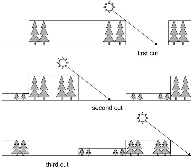
Figure 12.8 Wall-and-step cutting used to remove forest in three cutting cycles while providing shade to control melt rates and minimize impacts on peak flows.
