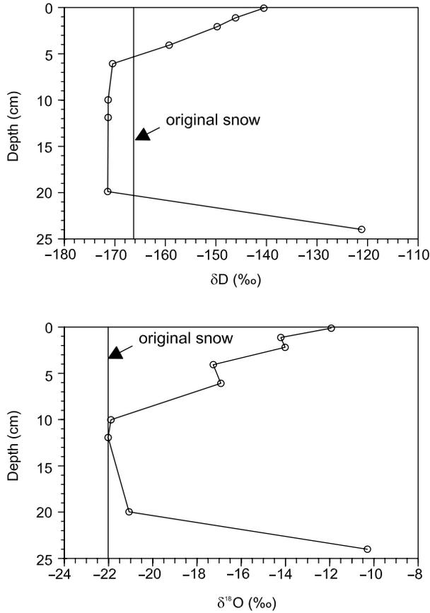
Figure 8.6 Isotopic profiles of  $\delta^2H$  and  $\delta^{18}O$  with depth in a snow column after 31 days of temperature gradient metamorphism showing enrichment in surface and bottom layers due to fractionation caused by vapor movement and sublimation (Cooper, 1998 after Sommerfield *et al.*, 1991, © 1991 with permission from Elsevier).
