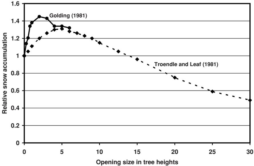
Figure 12.4 Maximum snow accumulation in conifer forest openings as a function of opening size, redrawn from Troendle and Leaf (1981) and Golding (1981). Opening size is measured in the downwind direction in multiples of tree height ( $H$ ).
