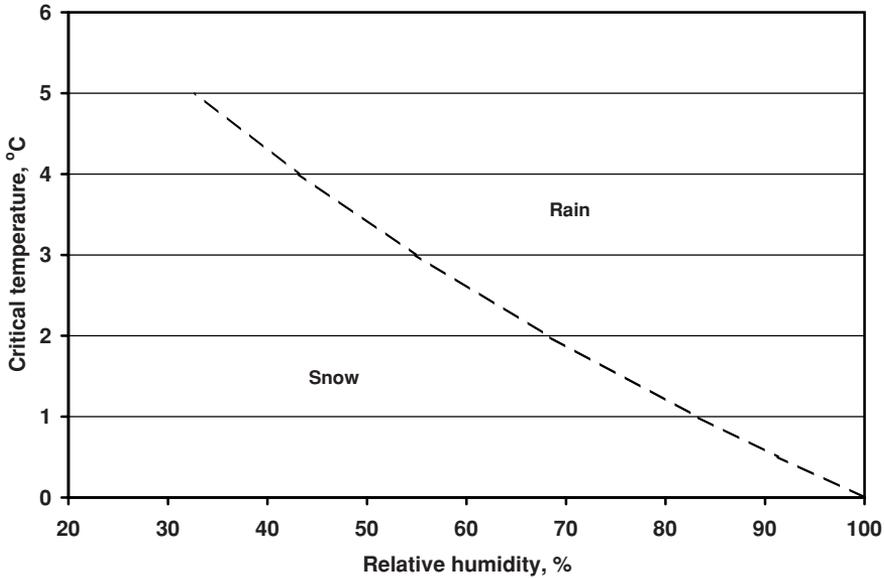
Figure 10.3 Critical temperature for separation of rain/snow events and maximum relative humidity conditions predicted with the psychrometric equation.
