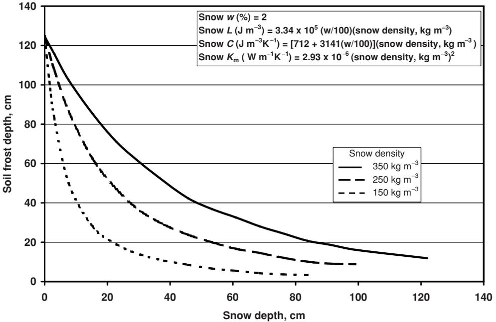
Figure 9.6 Computed relationship between seasonal soil frost depth and depth of snow cover for three snowpack densities. Calculations were based upon a trial-and-error method for the modified Berggren equation given by Aldrich (1956) for soil and climatic conditions used in the text example and snow properties given in the figure.
