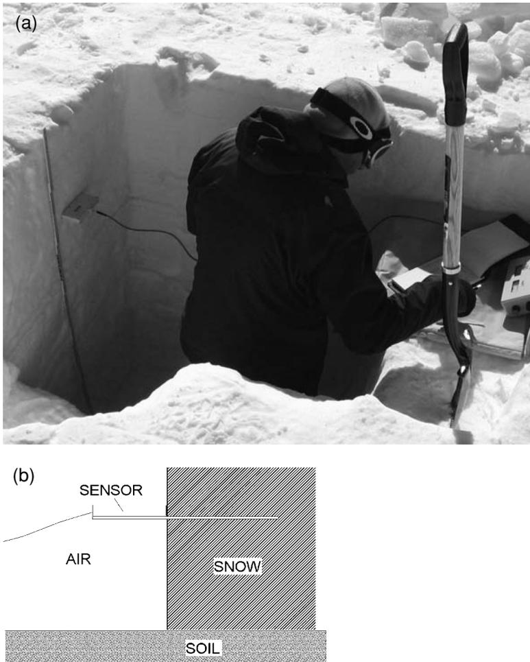
Figure 4.10 Capacitance probe/dielectric device being used on the Devon Ice Cap, Nunavut, Canada (a) to measure snow wetness. Bottom diagram (b) shows the so-called “Denoth probe” inserted into a snow pit wall (photograph courtesy J. Sekerka, and M. Demuth, Geological Survey of Canada; drawing adapted from Østrem and Brugman, 1991).
