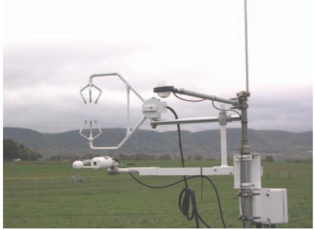
Figure 6.5 Solar-powered climate stations equipped with data loggers (left) are used to provide data (wind speed, air temperature, humidity) to support computations of snowpack convective exchange. The addition to climate stations of sonic anemometers (top right), fine-wire thermocouples, and high-speed open-path gas analyzers for CO<sub>2</sub> and water vapor (bottom right) allows computation of convective exchange using the eddy covariance method (photographs by D. DeWalle).
