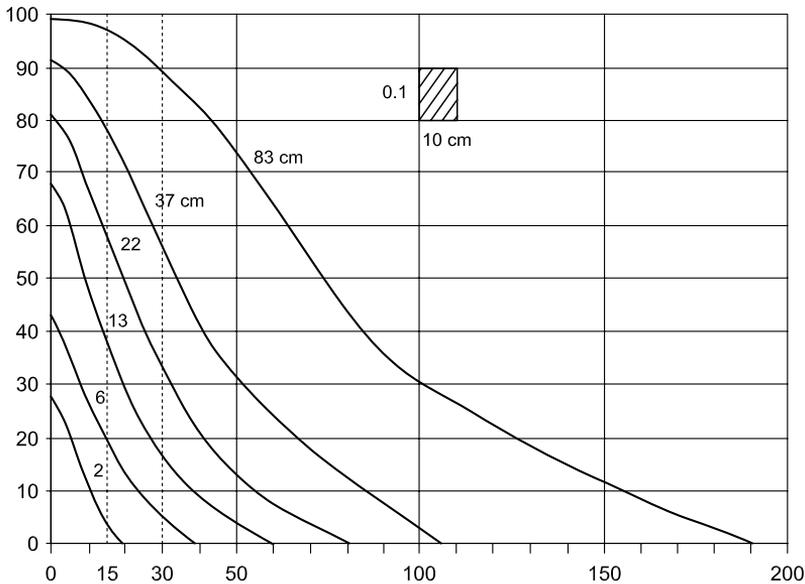
Figure 11.16 Nomograph of modified depletion curves for the elevation zone B (1284 km<sup>2</sup>, 2926–3353 m a.s.l.) of the Rio Grande basin. The curves are labelled with the areal average water equivalent (April 1) of the snow cover which they represent (Rango and van Katwijk, 1990).
