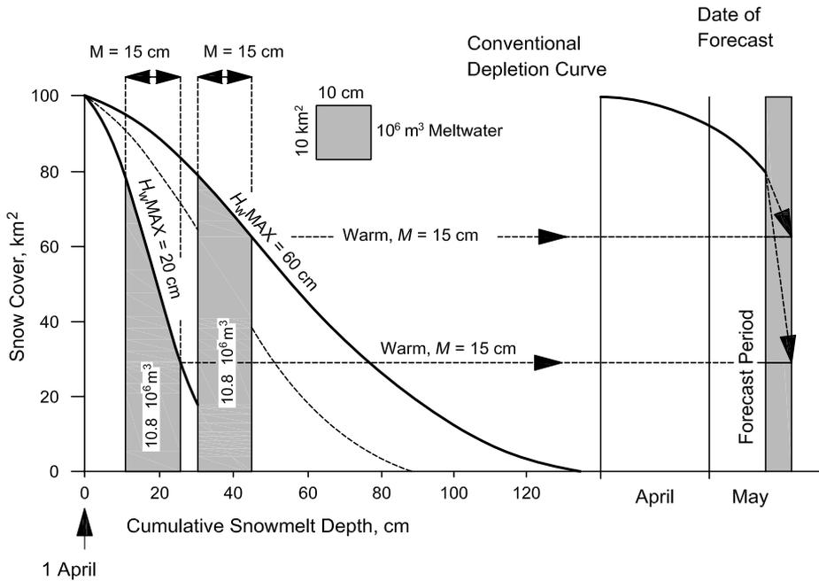
Figure 11.15 Extrapolation of snow-cover depletion curves in real-time from modified depletion curves with the use of temperature forecasts.  $H_{W\ MAX}$  is the water equivalent of the snow cover at the beginning of the snowmelt season (courtesy D. Hall and J. Martinec).
