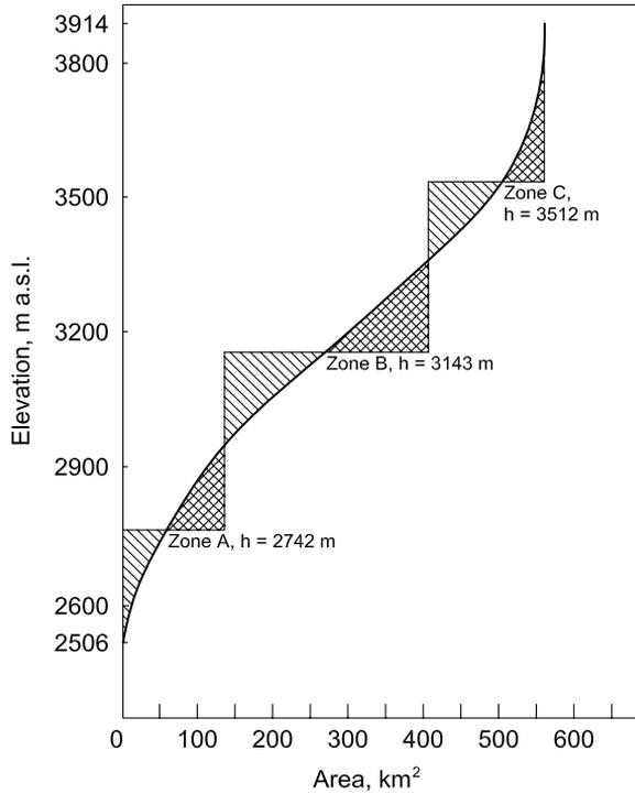
Figure 11.3 Determination of zonal mean hypsometric elevations ( $\bar{h}$ ) using an area–elevation curve for the South Fork of the Rio Grande basin.
