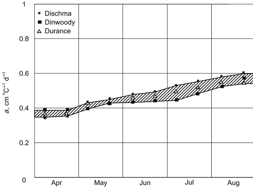
Figure 11.8 Average degree-day ratio ( $a$ ) used in runoff simulations by the SRM model in the basins Dischma (10 years), Durance (five years) and Dinwoody (228 km<sup>2</sup>; 1981–4202 m a.s.l., Wyoming, 2 years) (Martinec and Rango, 1986).
