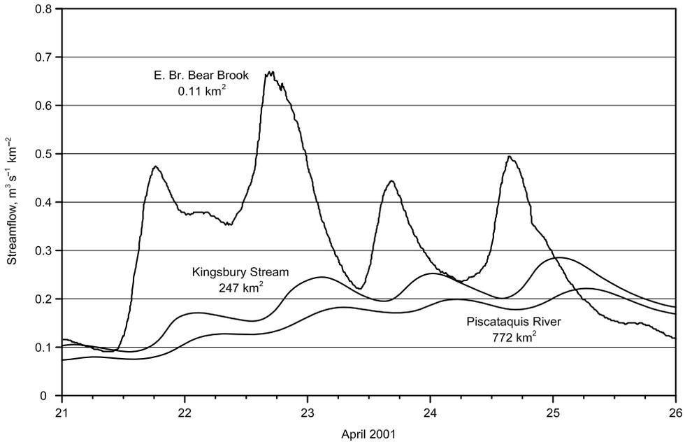
Figure 9.8 Comparison of timing of daily streamflow hydrographs during snowmelt on April 21–25, 2001 for three basins with varying area in Maine, <http://water.usgs.gov/realtime.html>.
