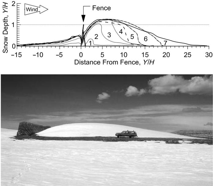
Figure 12.1 Stages of snow-drift growth upwind and downwind from a 50% porosity Wyoming snow fence. Drift depth and length are scaled to fence height ( $H$ ). (Tabler, 2003, © 2003 by Ronald D. Tabler, all rights reserved. Reprinted with permission).
