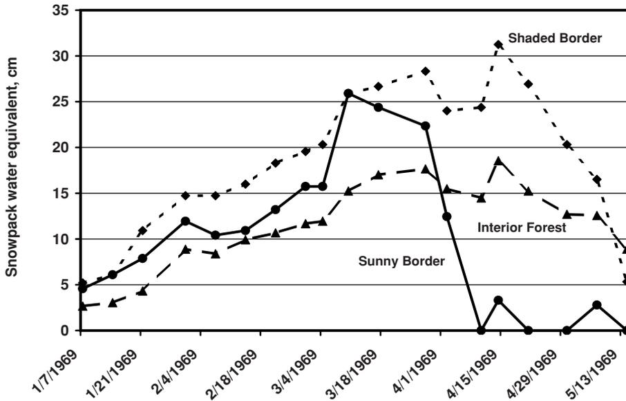
Figure 12.6 Snow accumulation and ablation patterns in interior forest and along the shaded and sunny border of a  $1H$  wide, E–W oriented clear-cut strip in Englemann spruce (*Picea engelmanni* Parry) forest in New Mexico (redrawn from Gary, 1974 courtesy USDA Forest Service).
