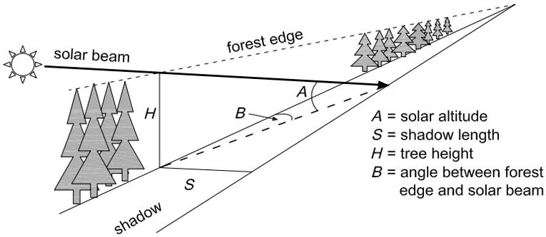
Figure 12.7 Shadow length–solar geometry relationships along infinite forest edge.
