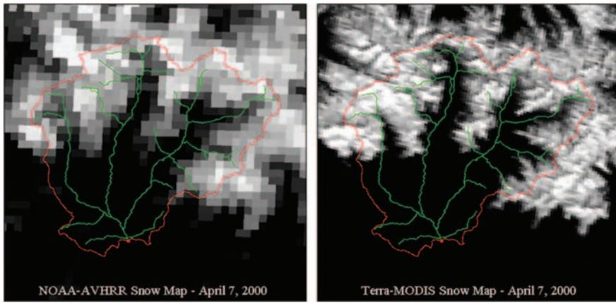
Figure 5.4 Comparison of NOAA-AVHRR and MODIS derived snow cover for the Noguera Ribagorzana Basin ( $572.9 \text{ km}^2$ ) in the Central Pyrenees of Spain on April 7, 2000. The different gray levels correspond to different percents of snow cover in each pixel. Snow cover in the Basin totals  $181 \text{ km}^2$  from AVHRR and  $184 \text{ km}^2$  from MODIS as reported by Rango *et al.* (2003).
