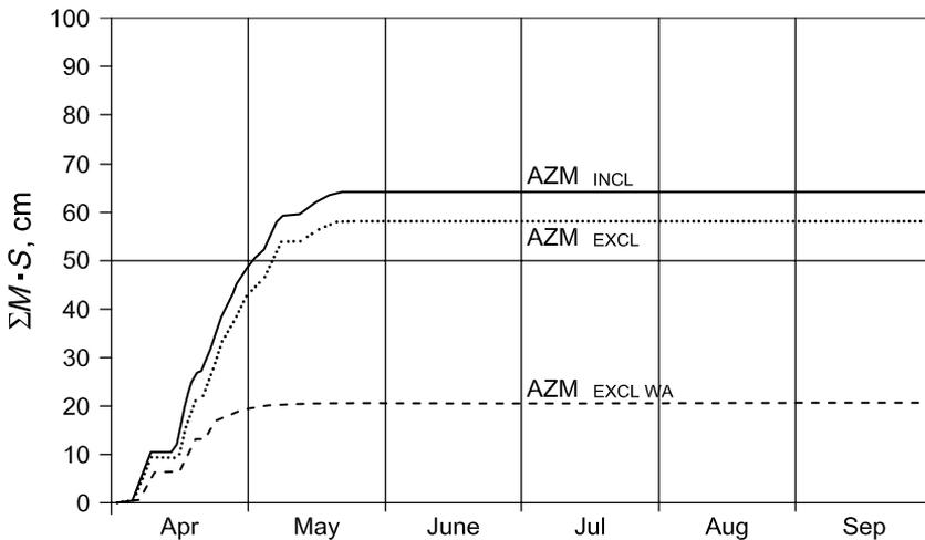
Figure 11.25 Accumulated zonal melt curves for zone A:  $AZM_{INCL}$ : computed daily melt depth multiplied by  $S$  from  $CDC$  (= zonal melt).  $AZM_{EXCL}$  with new snow zonal melt excluded and  $AZM_{EXCL WA}$  derived from  $AZM_{EXCL}$  by cutting it off on April 27 and transferring it to April 1.
