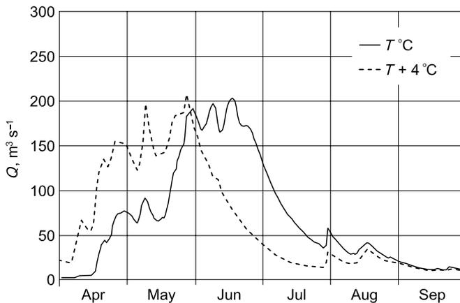
Figure 11.28 Climate-affected runoff ( $T + 4^\circ C$ ) in the Rio Grande basin near Del Norte, compared with the runoff simulated by data of 1979 (as shown in Figure 11.22) for April–September.
