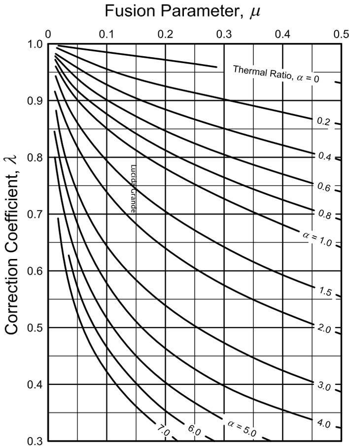
Figure 9.5 Dimensionless parameter  $\lambda$  used in the modified Berggren formula to compute the depth of soil frost (Aldrich, 1956, Transportation Research Board, National Research Council, Washington, DC, Figure 5, p. 133. Reprinted with permission of TRB).
