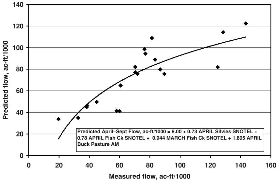
Figure 10.1 Example of a working equation used to predict total April–September streamflow for the Donner und Blitzen River in southeastern Oregon USA based upon snowpack-water-equivalent (SNOTEL) and snow-depth aerial-marker (AM) data (courtesy USDA NRCS National Water and Climate Center).
