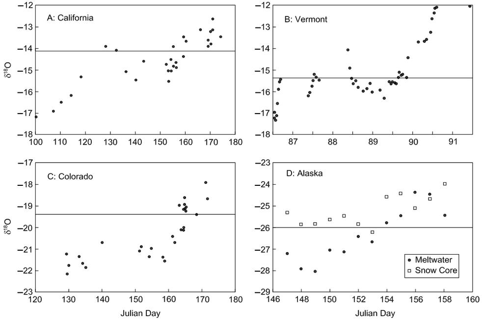
Figure 8.7 Progressive changes in meltwater  $\delta^{18}\text{O}$  during the melt season at four US sites showing depletion in early melt followed by enrichment in later melt relative to the original snowpack condition (horizontal line) (Taylor *et al.*, 2002, © 2002 with permission from John Wiley and Sons).
