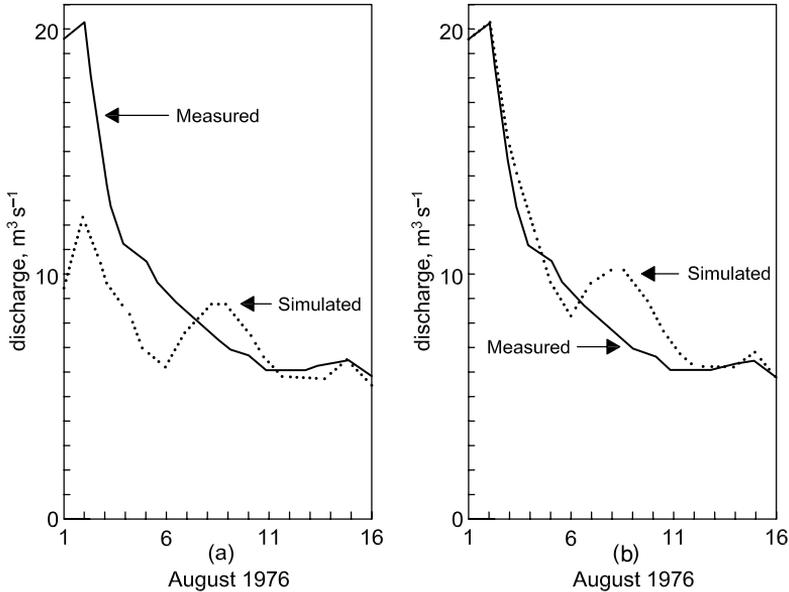
Figure 11.19 Discharge simulation in the Dinwoody Creek basin (228 km<sup>2</sup>, 1981–4202 m a.s.l.) in Wyoming, (a) without updating, and (b) with updating by actual discharge on August 1.
