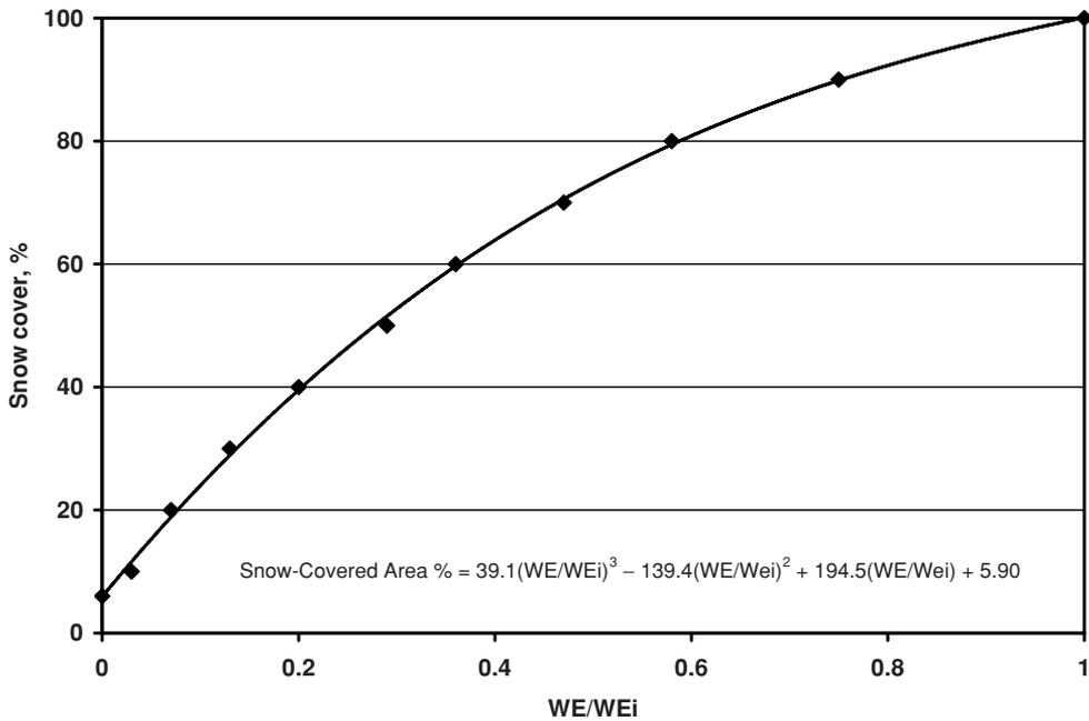
Figure 10.7 Generic snow-cover depletion curve used to relate snow-covered area on a watershed (%) to a snowpack-water-equivalent index ( $WE/WE_i$ ) (based upon Anderson, 1976);  $WE$  = snowpack water equivalent and  $WE_i$  = minimum snowpack water equivalent where snow-cover area always equals or exceeds 100% on a basin.
