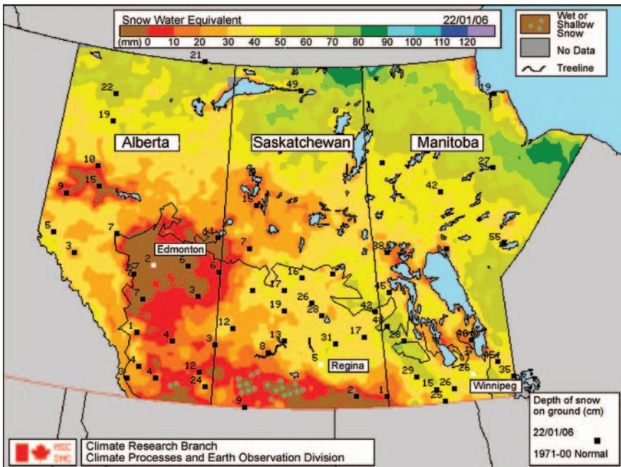
Figure 5.3 Operational snow-water-equivalent map for the Canadian Prairies on January 22, 2006 derived from passive-microwave satellite data. Numbers on the map indicate point measurements of observed snow depth. Maps are distributed by posting on the World Wide Web, [www.socc.ca/SWE/snow'swe.html/](http://www.socc.ca/SWE/snow'swe.html/). (Reproduced with the permission of the Minister of Public Works and Government Services Canada, 2006.)
